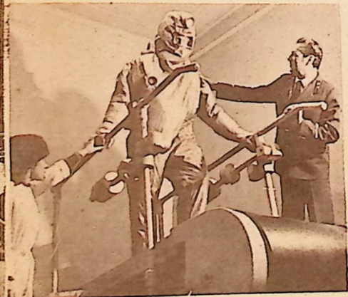
Testing to see how worker can perform on the job, when wearing a new "comfort" suit that keeps a man cool even in extremely high temperature operations.
